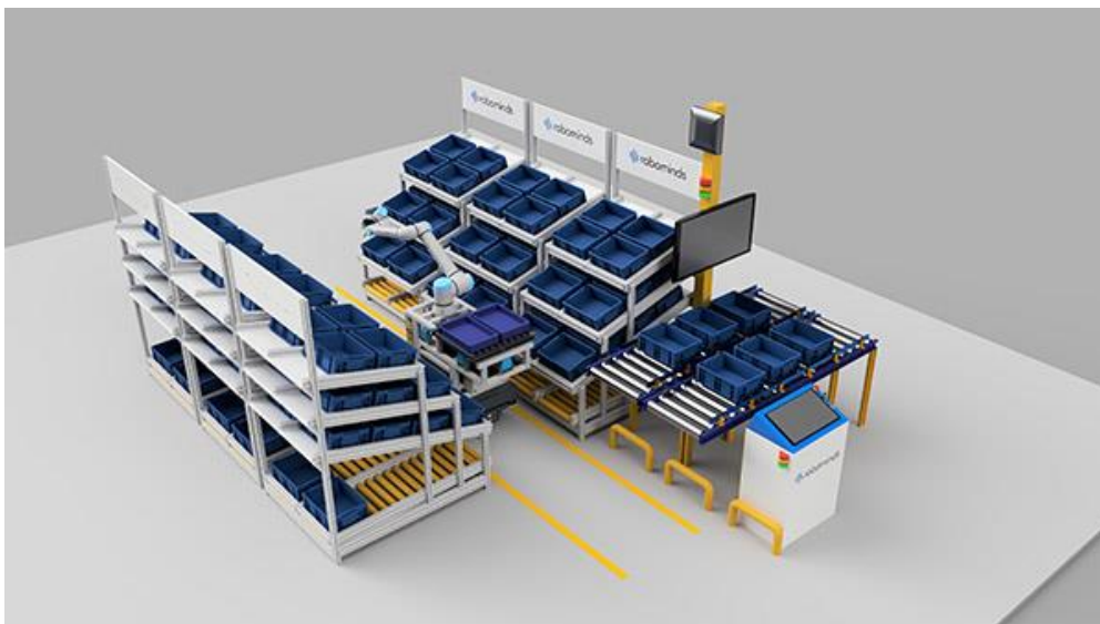
Figure 4. Robominds GmbH. Automated Kitting Station
