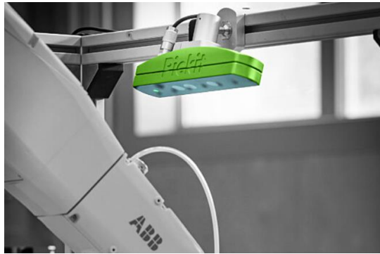
Figure 11. Pickit3D. Vision System for Bin Picking
