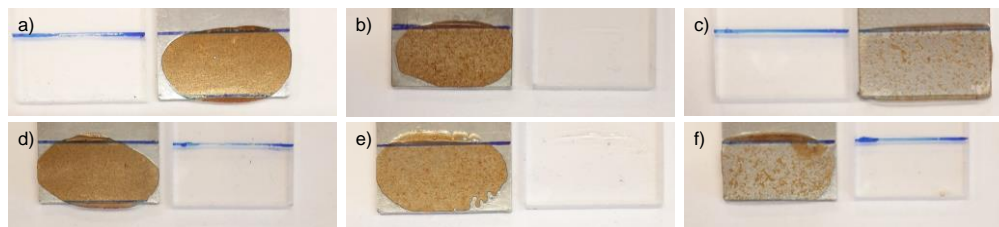
Figure A-II.19. Adhesive failure from the PMMA substrate of a) 70/30, b) 50/50 and c) 30/70 A-PHU/TMPTMP equivalent ratio formulations tested after 24 h at room temperature and d) 70/30, e) 50/50 and f) 30/70 equivalent ratio compositions tested after 1 week at the same conditions.
