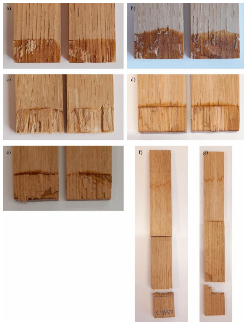
Figure A-II.15. Photos of the representative failure nature on oak wood substrates of the neat and doped (+3.9 mol% DOP and APTMS) 70/30 molar ratio aromatic diamine-based compositions depending on the surface treatment applied. a) Surface treatment A; b) Surface treatment B; c) Surface treatment C and d) Surface treatment C' for substrates glued with the neat composition; e) substrate glued with doped composition after surface treatment C'; substrate failure out from gluing line: f) neat composition, surface treatment C'; and g) dope formulation, surface treatment C'. Surface treatment: A wood was sanded with sandpaper and wiped with a paper wet in acetone; B surface treatment A + (5' in a mixture 1/1 acetone/isopropanol + 2' in water) x3 as reported elsewhere; 38 C surface treatment B + 1 night at 70 °C; C' surface treatment C + more quantity of adhesive (~80 mg).
