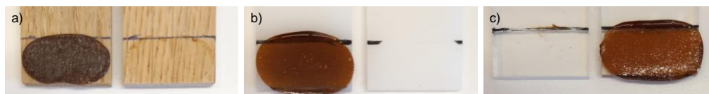
Figure A-II.41. Photos of the representative adhesion failure after lap-shear tests of 50/50-MXDA when it was applied onto a) oak, b) PE-HD and c) PMMA.
