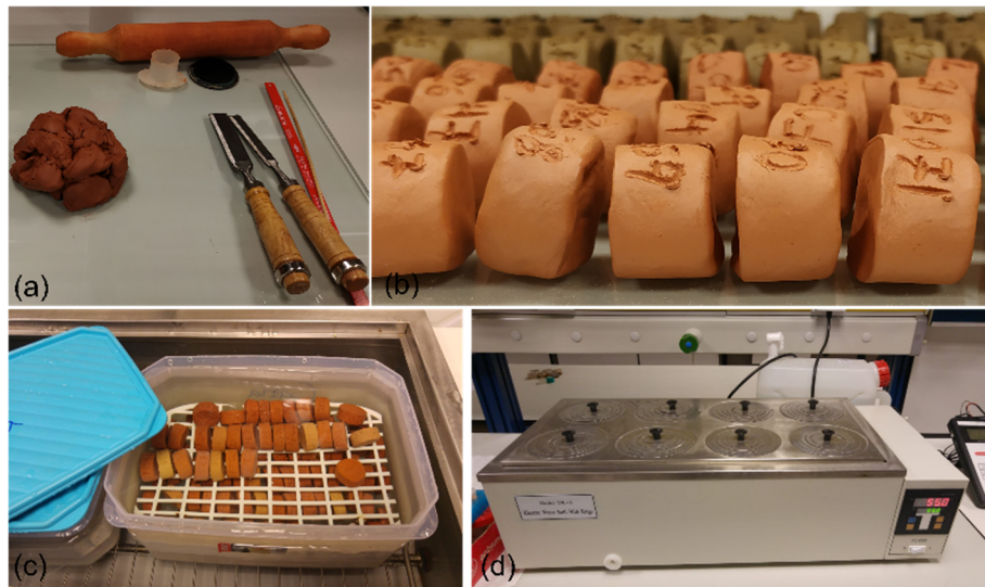
Figure 4.8. The manufacturing process of the test- and control-pieces before being fired: (a) the clay; (b) pieces before being fired; (c) test-pieces inside a seawater environment container; (d) the electric water bath containing the two containers with different environments (tap and seawater)
