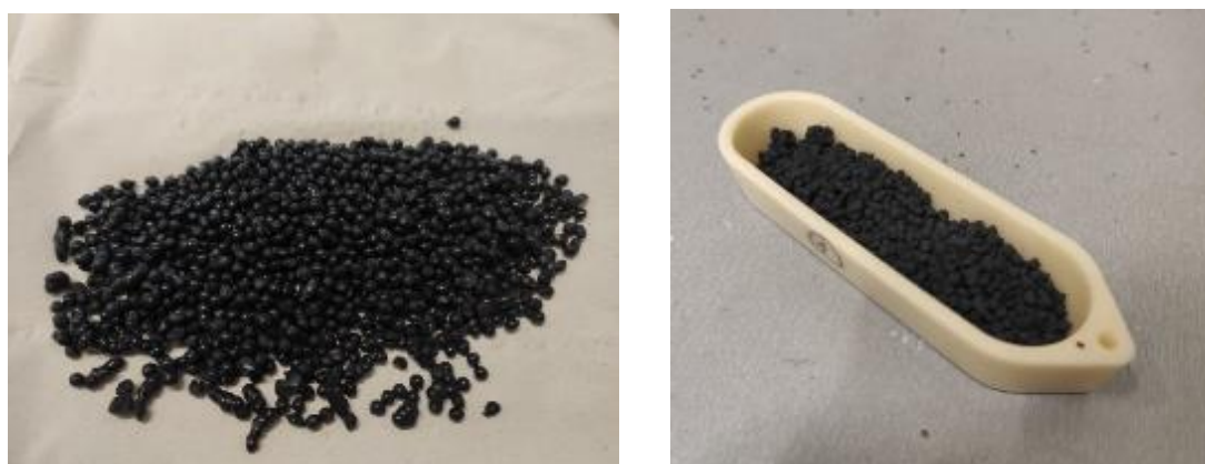
Figure 85. Mn 2 O 3 Si-doped granules 50:50 (MO:PB) for reactor testing: a) After step 2 of the synthesis route and b) After hardening at 1050°C for 4 h.
