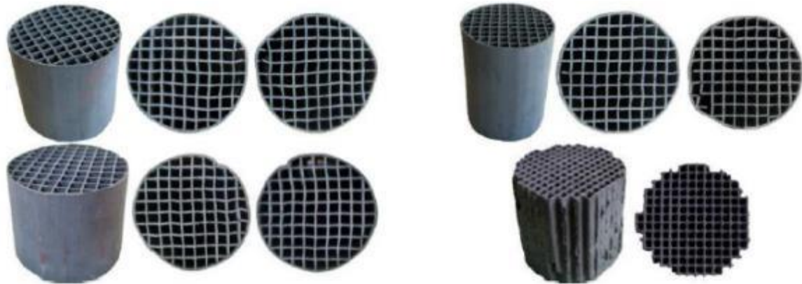
Figure 11. Honeycomb extrusion and coated structures of \text{Co}_2\text{O}_3 in the Center for Research and Technology-Hellas [59]. Copyright Elsevier 2015
