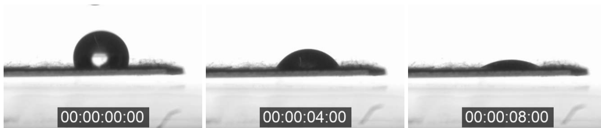
Figure 4.5. Absorption of a water droplet on a PVDF+PANI fiber mat, at 4 second intervals
