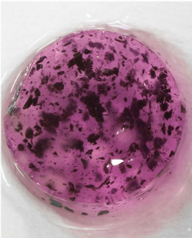
Hydrogel disk with magnetolectric microspheres.
