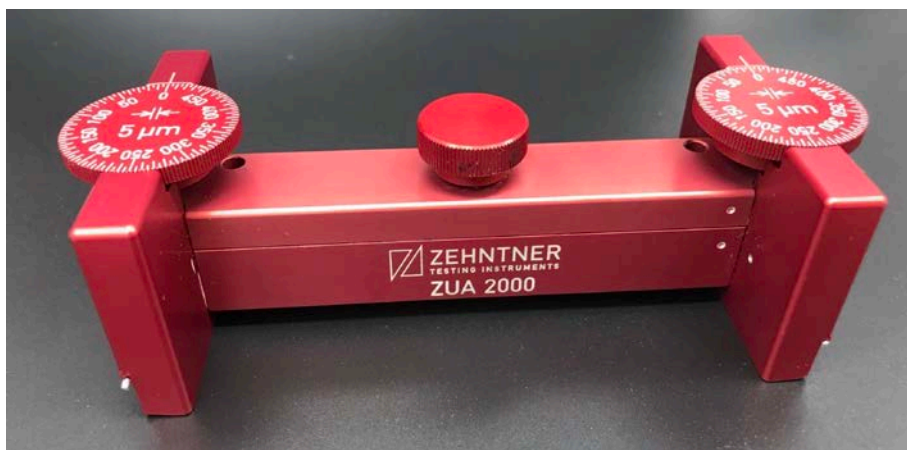
Figure 1.10. Photograph of a thickness-adjustable doctor blade.
