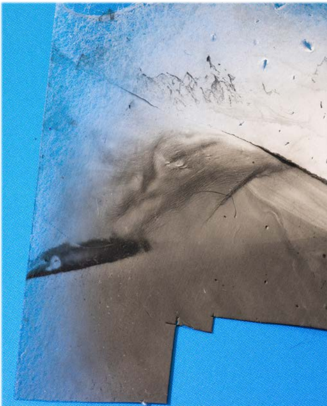
Conductive polymer coating on white electrospun polymer microfibers.
