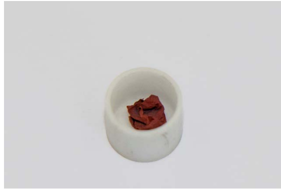
Figure 3.8. Remaining char after TGA analysis of a PVDF+Fe 3 O 4 15% fiber sample.
