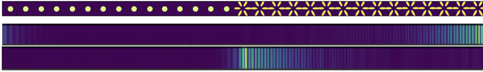
FIGURE 5.9: Upper panel shows the ribbon structure composed by a trivial phase and a topologically fragile phase. Both lower panels correspond to the degenerate modes that exit within the gap.
