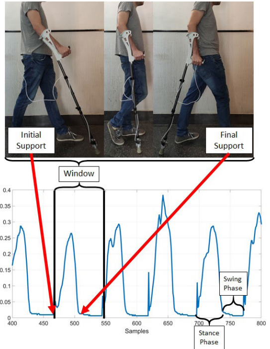
FIGURE 3. Cycle of use of an ADW and its phases. Data Segmentation in windows by using the data acquired from the force sensor.
