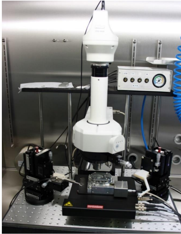
Figure 4.2: Transfer system and optical microscope. On the left and right of the microscope with large working distance objectives, two motor-controlled arms for holding the glass slide and micromanipulator can be seen. The stage has an integrated hotplate and can be rotated.
