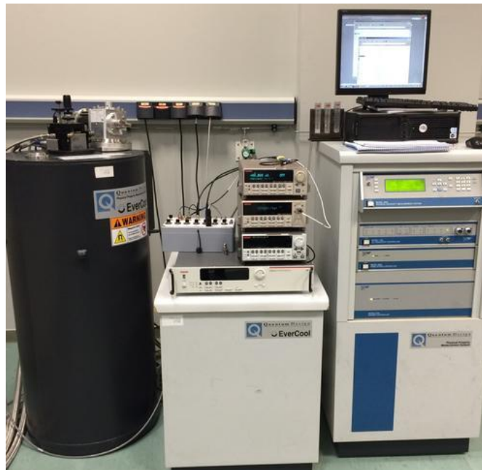
Figure 4.6: Physical properties measurement system. On the left, the Dewar of the cryostat is visible, in which vacuum shields the liquid helium that cools the sample. The temperature and the field of the superconducting magnets are controlled with the rack on the right. In the middle, the switch box for electrical contacts and the nanovoltmeter, the current source, and the source measure unit can be seen.
