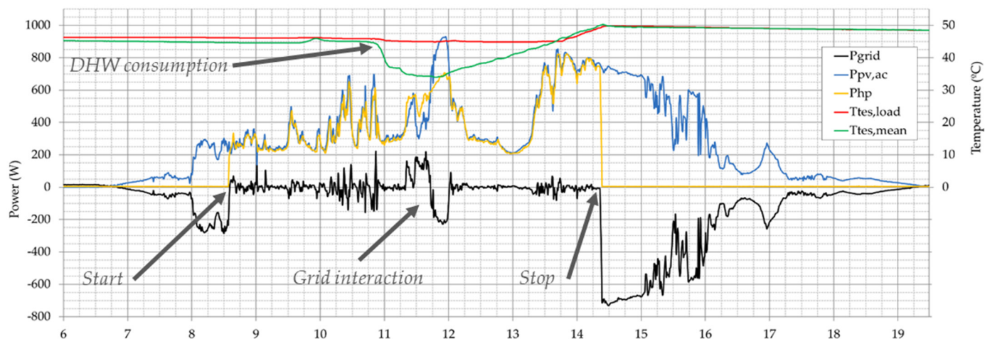
Figure 6. Main system electric power and TES state of charge profiles for the 15 April.
