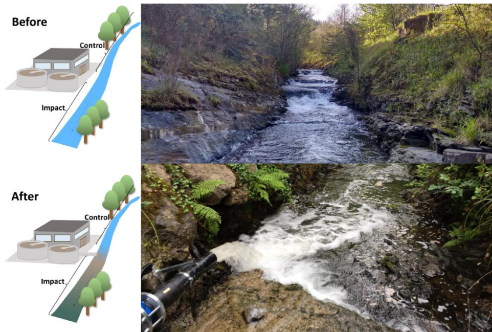
Fig. 2. Conceptual figure of the BACI (Before-After-Control-Impact) experimental design. The Control reach is upstream from the effluent pouring location. The Impact reach receives treated effluent during the After period. Photographs show the Control Reach and the effluent pouring pipe during a release occasion. Photographs are provided by Miren Barrado and Arturo Elosegi.
