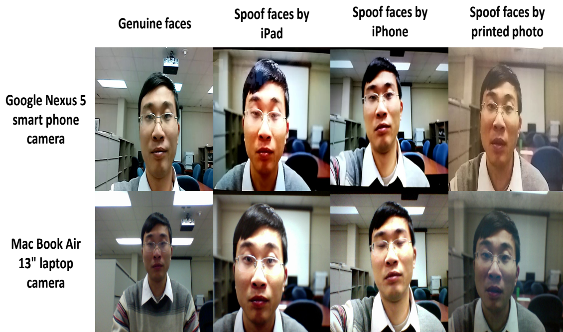
Figure 5. Example images of genuine and attack presentation of one of the subjects in the MSU-MFSD database.
