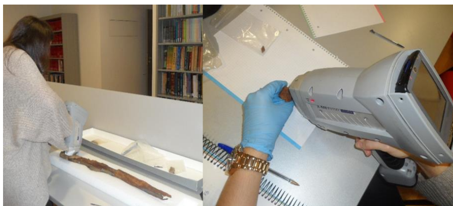
Figure 9 - Handheld XRF equipment fully operational
