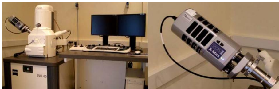
Figure 12 - On the left, SEM-EDS system with and EDS detail on the right
