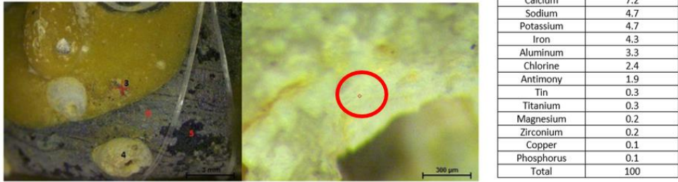
Figure 61 – Punctual analysis of the white points of the piece no.2 in the face A
