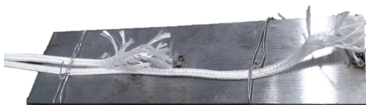
Figure 19. Sheet of the 2Mn steel prepared to carry out Q&P thermal treatment in furnaces and salt baths with one thermocouple welded in the center and other in the edge. The dimensions of the showed sheet were 250 mm length, 50 mm wide, and 1.5 mm thick.
