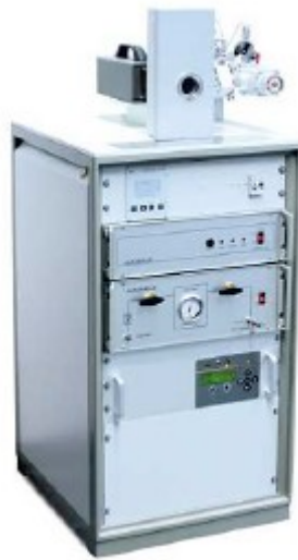
Figure 13. Global view on L78 RITA dilatometer.
