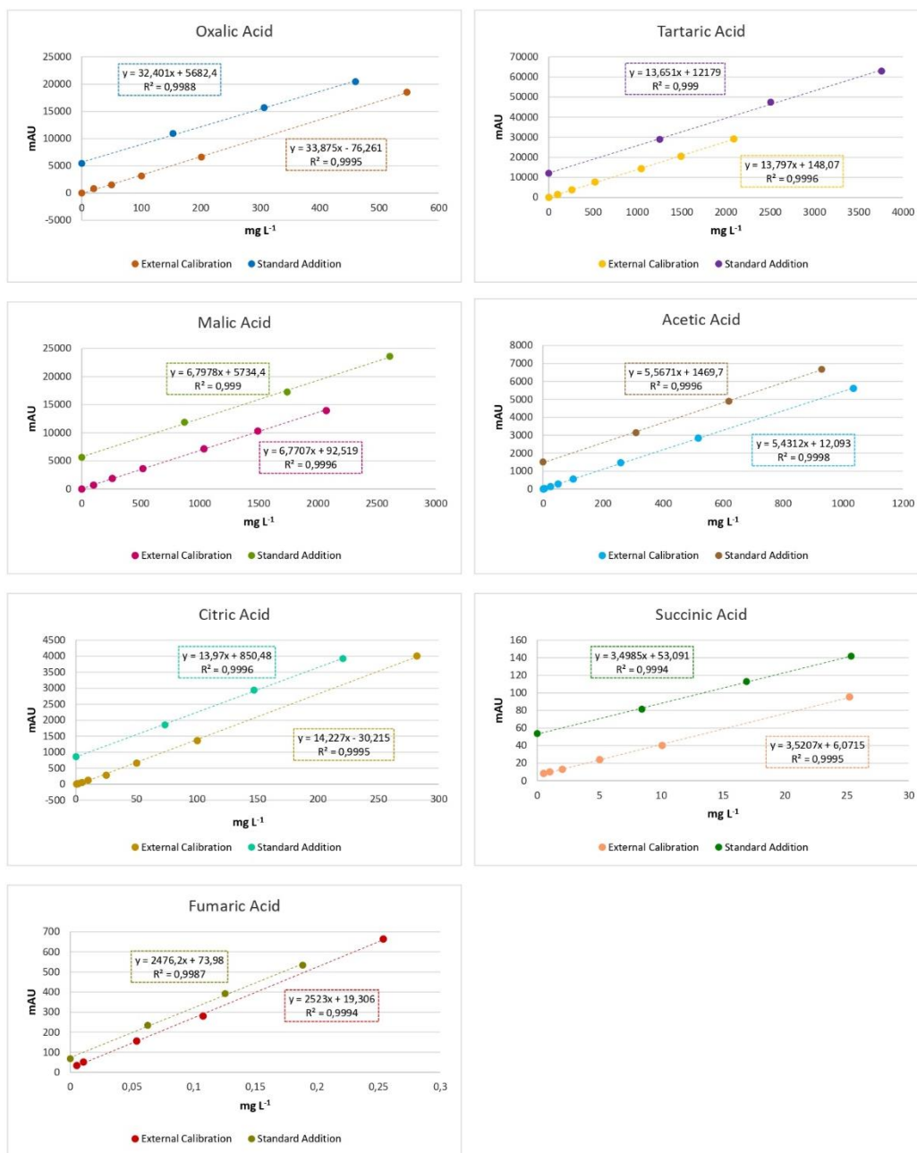
Figure IV.1. Matrix effect for Oxalic acid (a), Tartaric acid (b), Malic acid (c), Acetic acid (d), Citric acid (e), Succinic acid (f) and Fumaric acid (g) in a pooled leaf of Vitis vinifera L.
