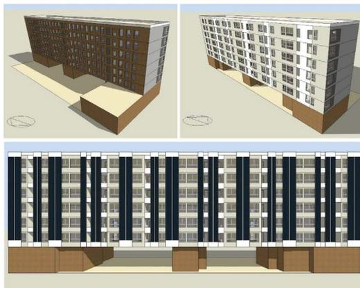
Fig. 10. Appearance of the building model for the two cases: North façade (upper left), south façade of the reference building (upper right) and of the building with PV-FVF (lower).
