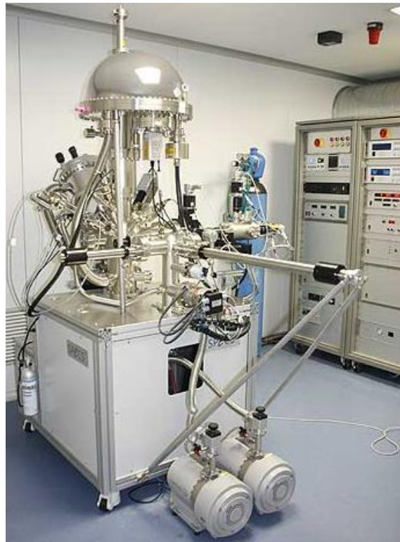
Figure A.2.9. SPECS system equipped with Phoibos 150 1D-DLD analyser.
