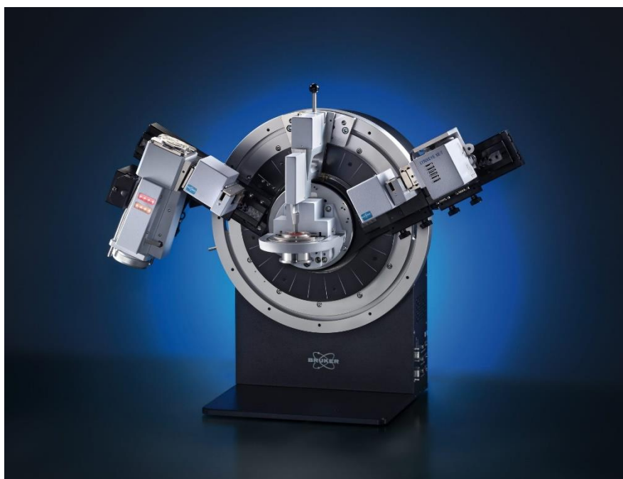
Figure 2.12. Bruker (D8 Advance) X-ray diffractometer picture [36].
