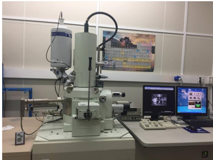
Figure 2.14. Scanning Electron Microscope MEB JEOL JSM-7000F at the SGiker of the University of the Basque Country (UPV/EHU).
