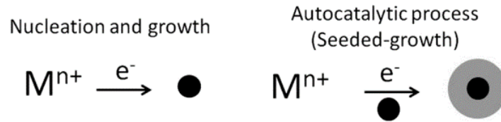
Figure 1.5.1: Two main mechanisms for the synthesis of gold nanoparticles. In the nucleation and growth mechanism, strong reducing agent reduces metal ions followed by growth into nanoparticles. In the seeded-growth process, autocatalytic reduction of metal ions takes place exclusively on the the surface of preformed seeds to produce particles of the desired shape and size. Reproduced from [32]
