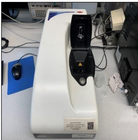
Figure 8: Picture of the DLS instrument used in this project: Malvern Zetasizer DLS.
