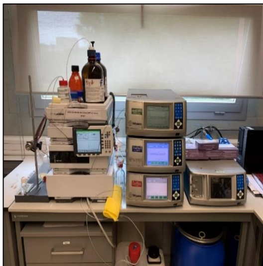
Figure 6: Picture of the 1200 Agilent chromatograph and different detectors used in this project.
