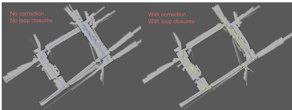
Figure 7.6: Importance of loop closures and pose corrections. The left image ignores pose correction, global loop closures and local loop closures. The right image is the map of the session.
