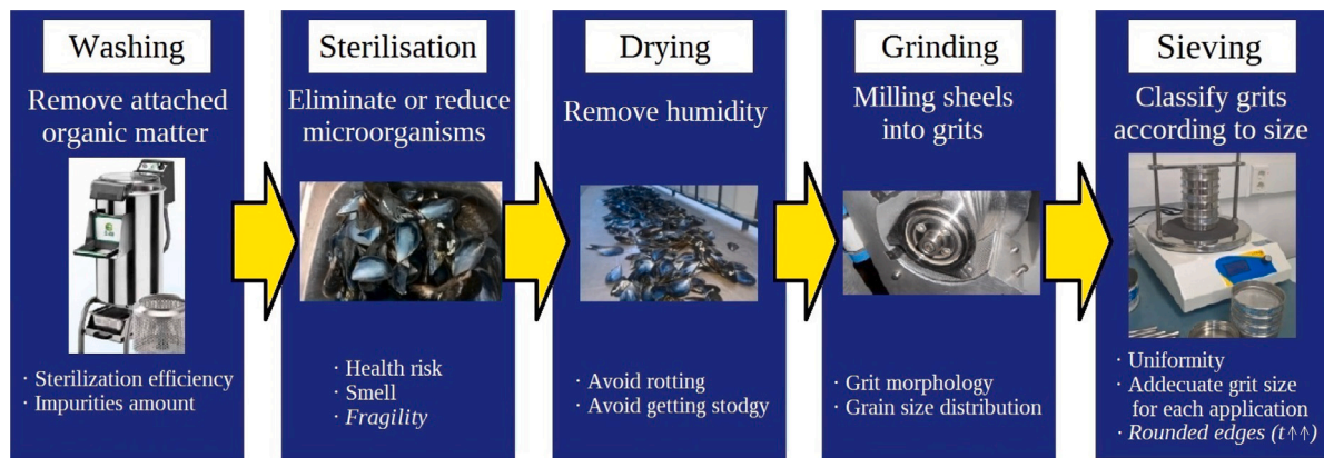
Fig. 1. Flow-chart of the steps to turn shells into abrasive sand. The effects and damage of the operation on the abrasive characteristics are listed below.
