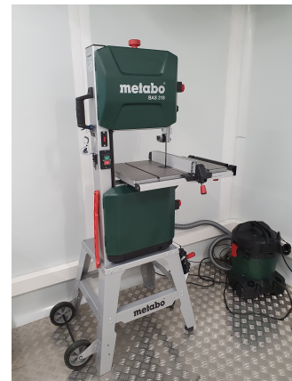
Figure 7: The vertical electric saw used at the IzotzaLab to cut ice. Approximate dimensions: 50x70x160 cm.
