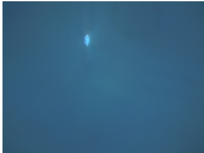
Figure 23: Bubble observed with the 63x immersion objective lens. The sample is illuminated with both incident and transmitted light. It is worth remembering that the width of the area in micrometers is provided in page 25.
