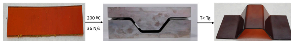
Figure 9. Validation of thermoforming capacity of aero grade epoxy vitrimer.
