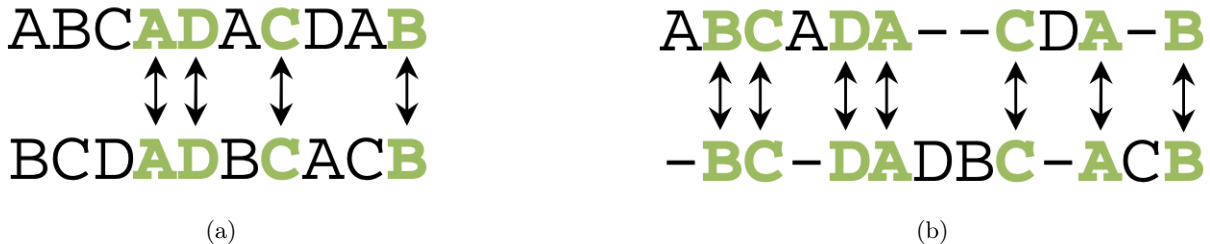
Figure 6: An example of the common subsequences of two sequences of character, (a) without inserting gaps between the characters (non-elastic) and (b) inserting gaps (elastic). When the gaps are inserted allowing elasticity, the number of common subsequences grows, as well as the size of some of such subsequences. Image taken from [21].
