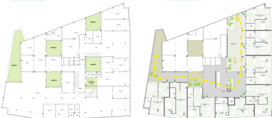
Figure 3. First Floor. Muro 16. a) Before, offices. b) After, apartments. New livingstyle and open courtyards. Authors of Proyecto de Ejecución. 2020.
