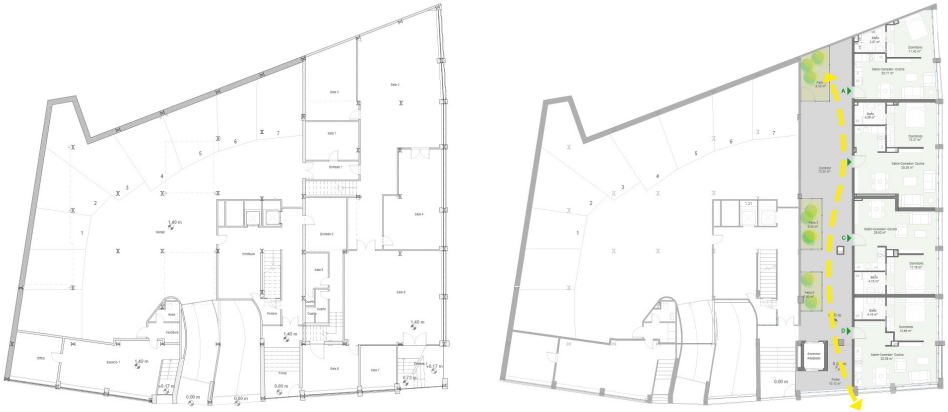
Figure 4. Ground Floor. Muro 16. a) Before, offices. b) After, apartments. New lifestyle and extended courtyards. Authors of Proyecto de Ejecución. 2020.
