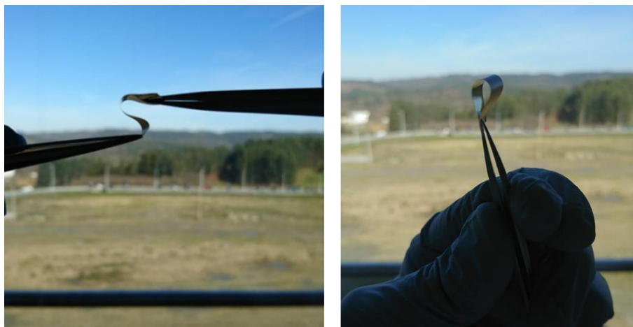
Figure 3.4. Optical photographs showing the bendability of NaCMC/CoFe 2 O 4 25wt.% nanocomposite films.
