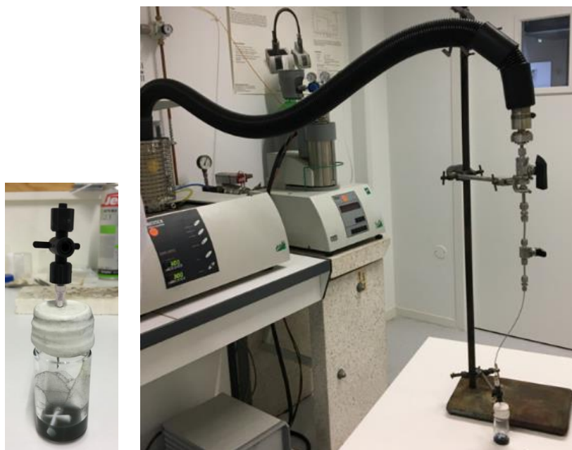
Figure A.9: Set-up for the mass spectrometry analysis of the gases released upon chemical oxidation of \text{Na}_3\text{V}(\text{PO}_3)_3\text{N} – the vial from the left photo was tightly connected to the Mass Spectrometer by the set of cables and valves, which were gradually opened upon the measurement.
