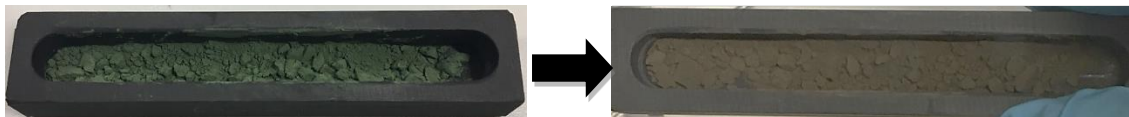
Figure 2.33: (left) powder of pristine \text{Na}_3\text{V}(\text{PO}_3)_3\text{N} before pressing into pellets; (right) powder of ionically exchanged \text{Li}_3\text{V}(\text{PO}_3)_3\text{N} obtained after grinding the pellets.
