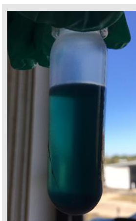
Figure 5.2: Image of the solution after microwave-assisted synthesis of \text{Na}_3\text{Li}_3\text{V}_2\text{F}_{12} .
