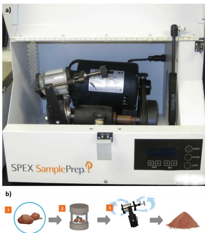
Figure A.11: (a) SPEX 8000M Grinding Ball miller; (b) SPEX ball mill mechanism with the back-and-forth shaking motion together with the lateral movements of the end of the jar. From SPEX SamplePrep 354
