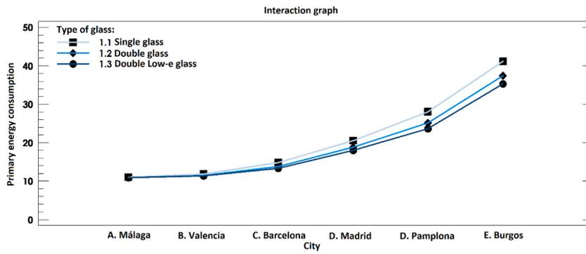
Fig. 6. Means of primary energy consumption ( $\text{kWh}\cdot\text{m}^{-2}\cdot\text{year}^{-1}$ ) obtained in each city depending on the type of glass used.
