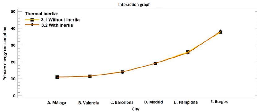
Fig. 9. Means of primary energy consumption (kWh·m<sup>-2</sup>·year<sup>-1</sup>) obtained in each city depending on the use of inertia.
