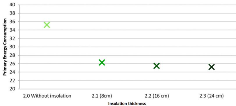
Fig. 7. Means of primary energy consumption ( $\text{kWh}\cdot\text{m}^{-2}\cdot\text{year}^{-1}$ ) obtained in Pamplona depending on the insulation thickness.
