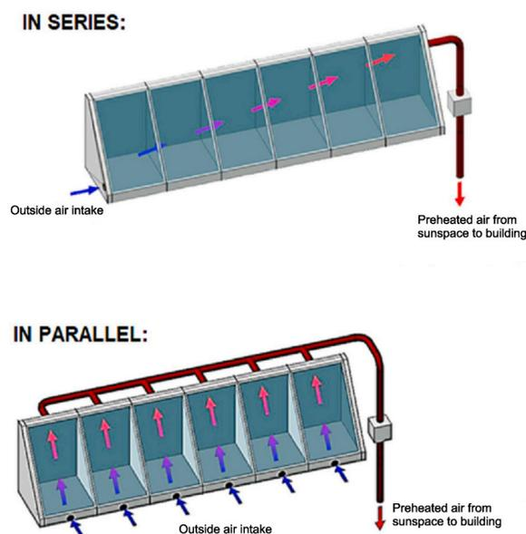
Fig. 1. Scheme of operation of the sunspace in series and in parallel.
