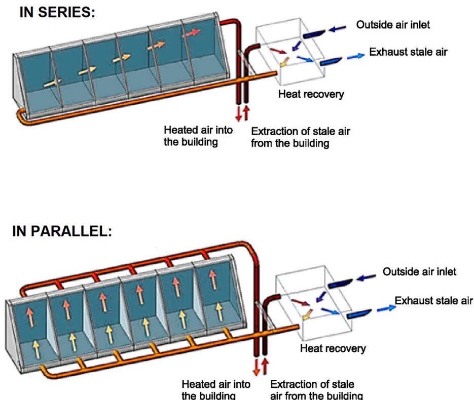
Fig. 2. Operation of sunspace in combination with a heat recovery ventilation system.
