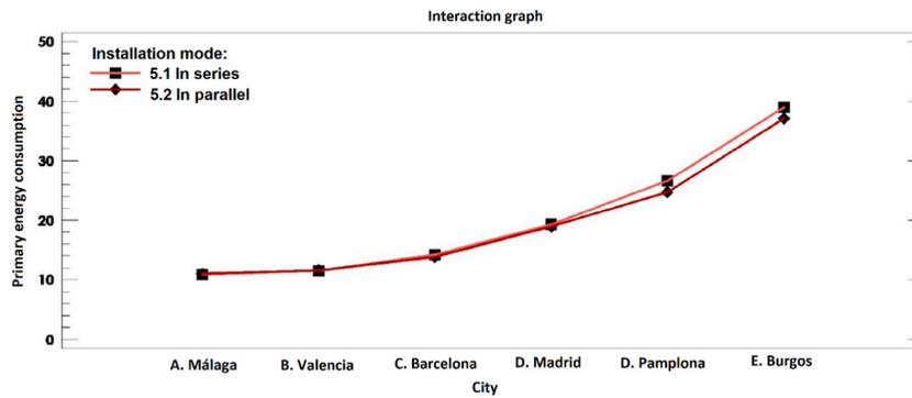
Fig. 12. Means of primary energy consumption (kWh·m<sup>-2</sup>·year<sup>-1</sup>) obtained in each city depending on the installation mode.
