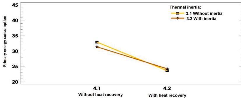
Fig. 10. Interaction graph between inertia and the use of heat recovery when the building is located in Pamplona.
