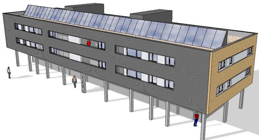
Fig. 5. Infographic of the building with the designed sunspace.
