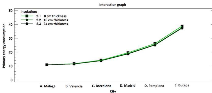
Fig. 8. Means of primary energy consumption ( $\text{kWh}\cdot\text{m}^{-2}\cdot\text{year}^{-1}$ ) obtained in each city depending on the insulation thickness.
