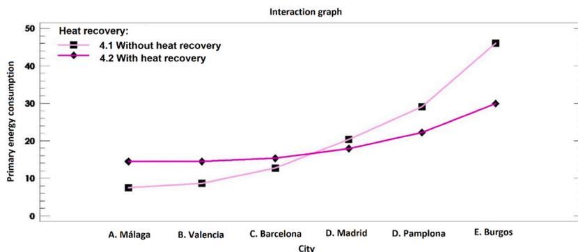
Fig. 11. Means of primary energy consumption (kWh·m<sup>-2</sup>·year<sup>-1</sup>) obtained in each city depending on the use of a heat recovery ventilation system.
