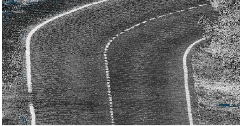
Figure 2.2: Intensity of the LiDAR sensor point cloud.
