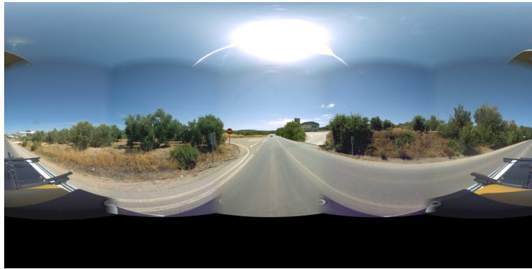
Figure 1.2: An example panorama from the ladybug sensor, obtained by the composition of the view of the five cameras.
