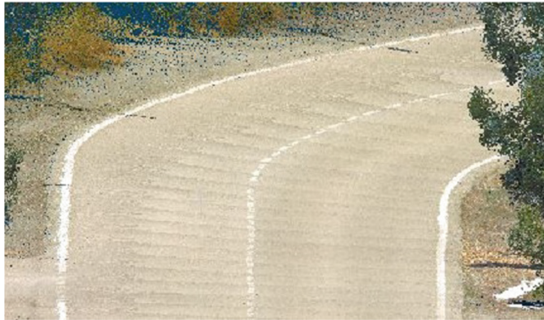
Figure 2.3: RGB image composed by the corresponding RGB pixels to each sample in the LiDAR point cloud.
