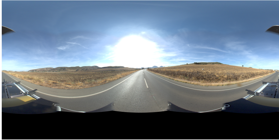
Figure 3.2: An example panorama image obtained from the ladybug sensor after stitching the 5 camera images, obtained by the composition of the views of the five cameras
