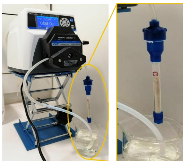
Figure 3.2. Image of the UiO-66-NH 2 /sand column experiment in closed circuit mode.
