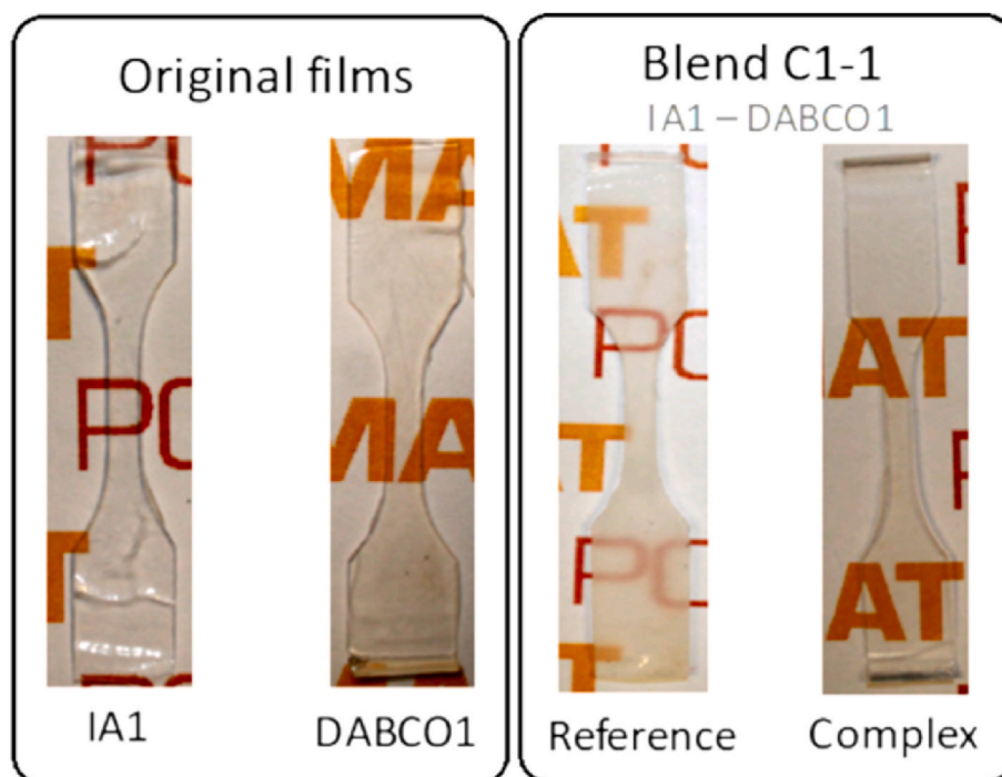
Fig. 4. Appearance of the individual polymers (IA1 and DABCO1) and the blend C1-1 films at different pH's (reference and ionic complex).
