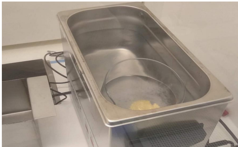
Figure 35. Lift off station
