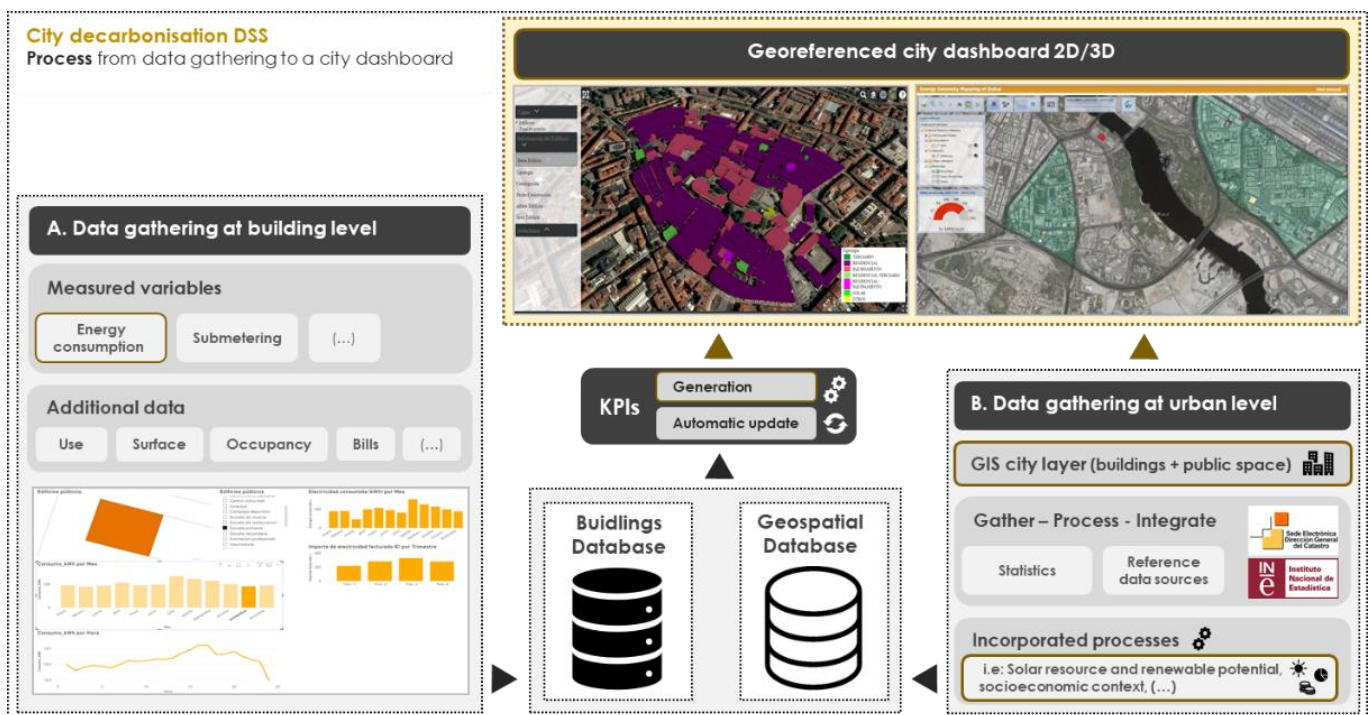
Figure 6. ENER-BI information flow: from data gathering at building and city level to a city dashboard
