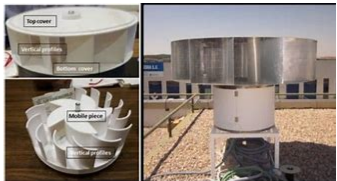
Fig. 1. View of the structure of the vertical axis wind turbine.
