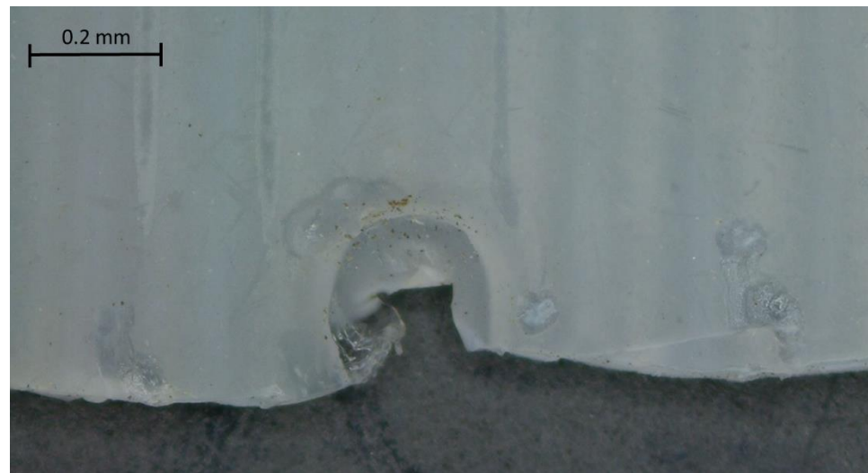
Figure 3. Chlorine-swollen pore causing premature failure.
