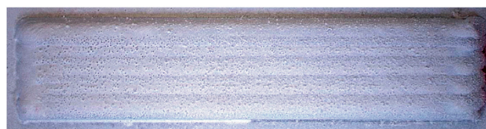
Figure 21. Reduction in crack sensitivity with the FGM strategy in Stellite 6 and WC MMCs. Adapted from [176].
