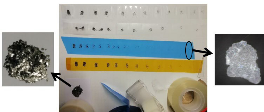
Figure 4. Natural graphite flakes' mechanical (physical) exfoliation to graphene many-layers by adhesive tapes (picture and microscope image are taken in Universidad del País Vasco- Euskal Herriko Unibertsitatea—UPV/EHU laboratories, Bilbao, Spain).
