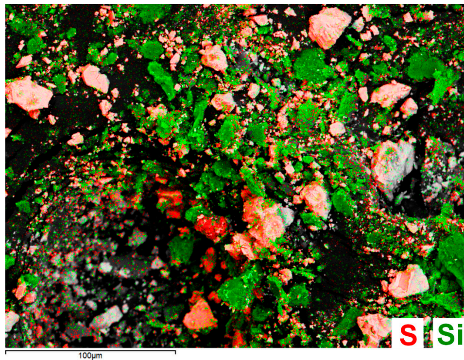
Figure 6. S and Si EDS maps acquired on the powdered mineral sample of Las Cuevas.
