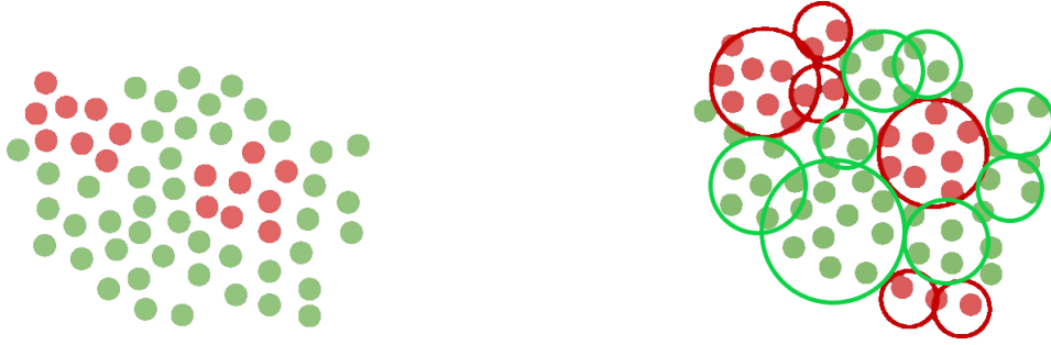
Figure 3: Different classes of point (red and green) in 2D space. On the right, the circles represent the radial basis functions mapped in the space according to the two point classes.
