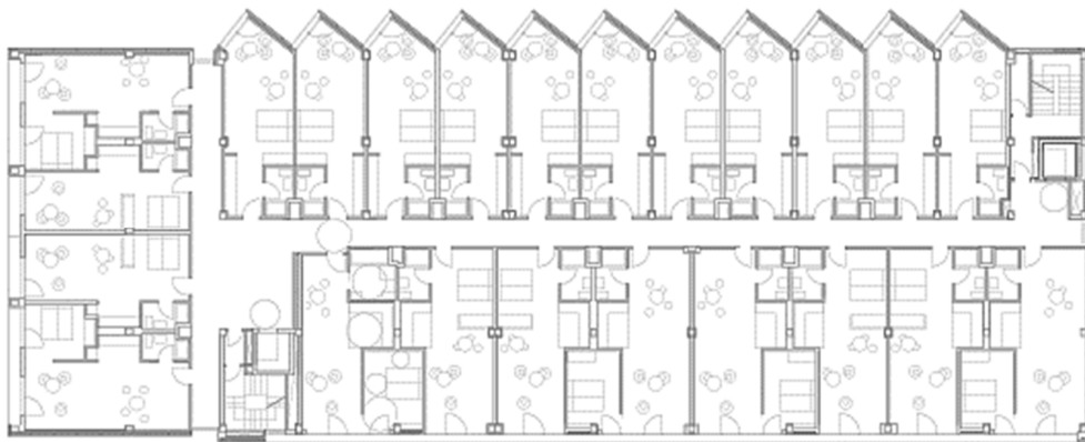
Figure 2. General floor plan of the project for 107 housing units in Txurdinaga by Oneka Arquitectura studio. Source: authors.
