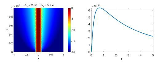
**Figure 2. Left** panel: time evolution of  $\log[\left|\psi_f(t,x)\right|^2]$  for the function with initial compact support  $f(x) = \cos^8(x/\Delta_x)$  (with  $\Delta_x = 1$  and  $p_0 = 0$ ) for short values of t. Note that the tails propagating beyond the light cone appear as soon as t > 0. **Right** panel: Fraction of that same wave packet outside the light cone, where the transient aspect can be noticed.
