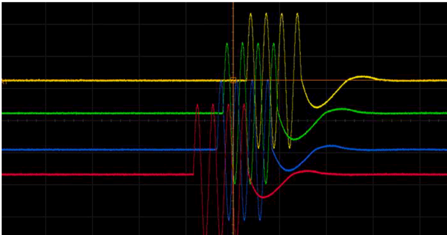
Fig. 4. Screen capture of the oscilloscope acquisition in the leads of four PWASs when 300 kHz waveform is applied (deflection factors 10 V/div and time base 5 \mu s/div). SHMUS output is configured with adjustable delays. The capture shows delays adjusted to 5.23 \mu s, 6.57 \mu s and 11.67 \mu s.
