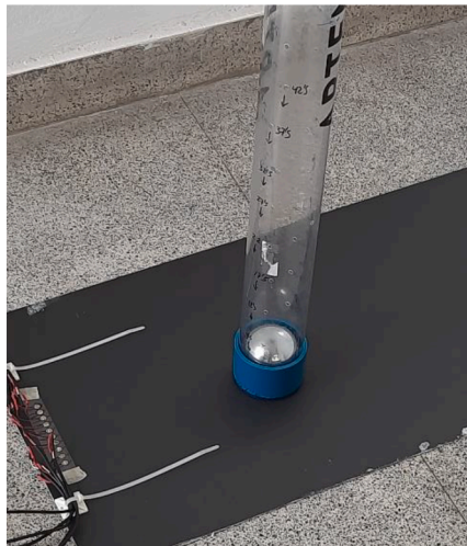
Fig. 9. Setup to produce controlled impacts on a CFRP board.
