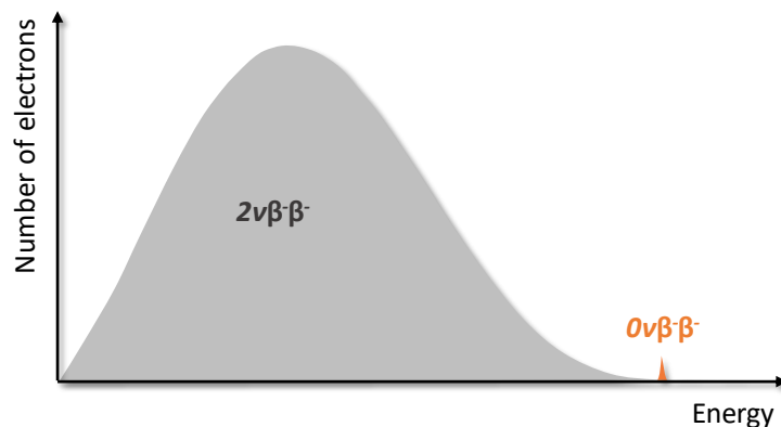
Figure 1.5. Energy difference of the electron produced in a 2\nu\beta\beta or 0\nu\beta\beta decay.
