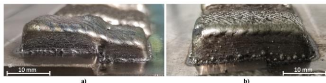
Fig. 6. Results of test specimen. a) Without dynamic control, b) with dynamic height and velocity percentage control.
