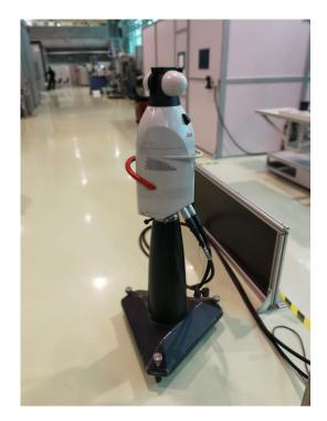
Fig. 3.1. – The laser tracker used to measure distances with a micrometric accuracy. It serves as ground truth to measure localisation errors.
