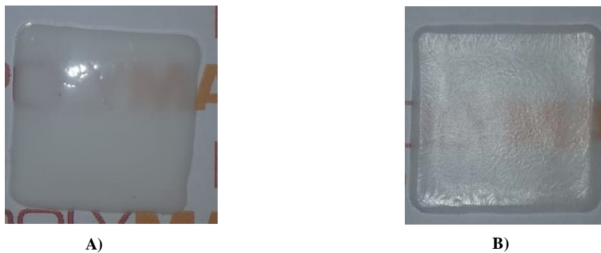
Figure I.6. Photos of the prepared film from A) the GDMA-DATP+TVCH based latex in silicone mold at 25°C and 55% of humidity B) the GDMA-DATP+TMPMP based latex in silicone mold at 25°C and 55% of humidity
