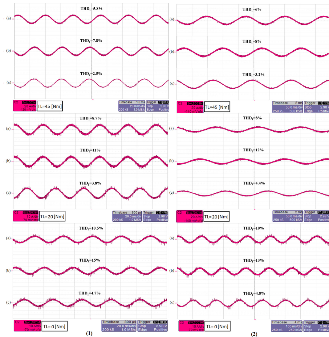
Fig. 11. Experimental results: Stator current performance at (1) 800[rpm] and (2) 200[rpm], with a different range of torque load, for (a) PCC_{z\beta} , (b) PCC_{dq} and (c) PCC_{dq-LPF} , at T_s = 12.5[\mu s](80[KHz]) .
