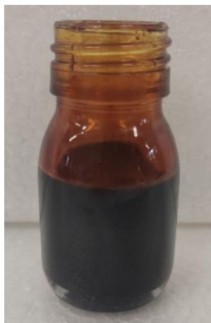
Figure 7.8. Glycolyzed mixture product obtained after the glycolysis of the synthesized thermoset PUs.
