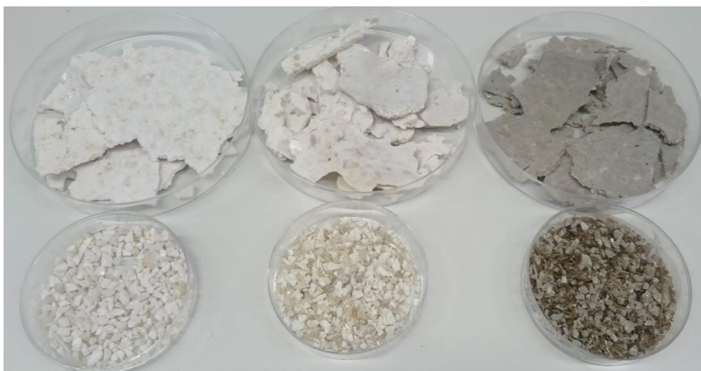
Figure 4.7. From left to right digital images of the compressed (at the top) and thermo-mechanically processed RPET-ssp, RPET-u and RPET-m samples.
