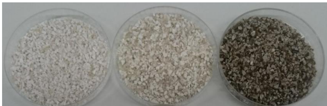
Figure 4.2. Samples shredded after thermo-mechanical recycling from left to right: RPET-ssp, RPET-u and RPET-m .
