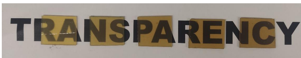
Figure 7.1. Thermoset PUs with increasing BHET-m content, from left to right.
