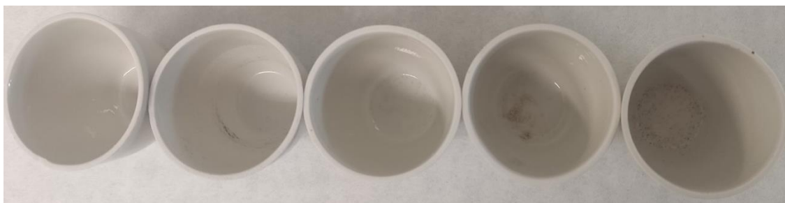
Figure 3.1. Ashes for PET-v, PET-ssp, PET-bottle, PET-m and PET-u from left to right.
