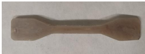
Figure 6.8. Injected RTPU sample obtained by thermo-mechanical recycling.
