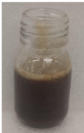
Figure 6.14. TPU-Gly obtained from the glycolysis reaction of TPUs.
