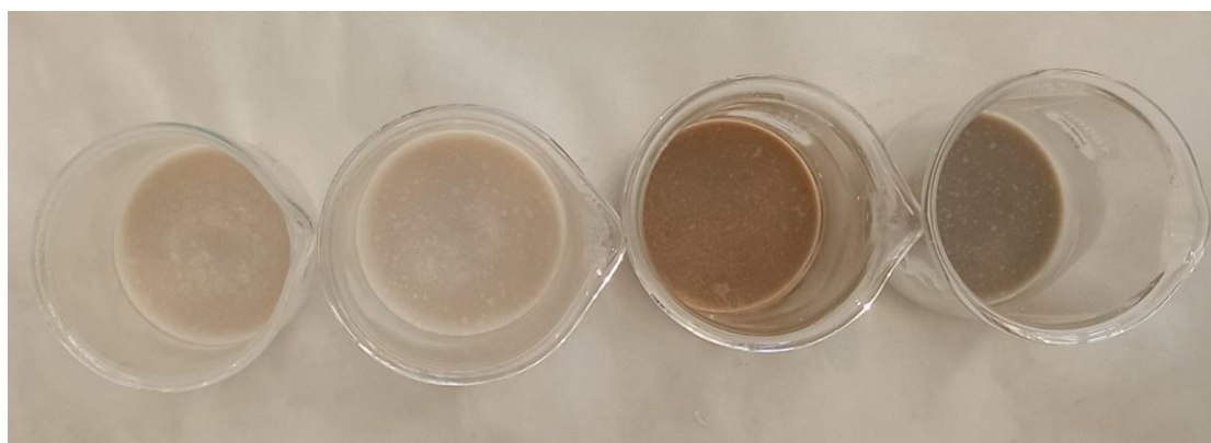
Figure 5.12. Digital image of the glycolysis products obtained from the depolymerization reactions of PET-v, PET-ssp, PET-u and PET-m (from the left to the right).
