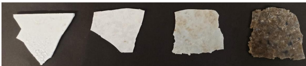
Figure 3.6. Images of PET samples obtained by compression molding. From left to right: PET-ssp, PET-v, PET-u and PET-m.
