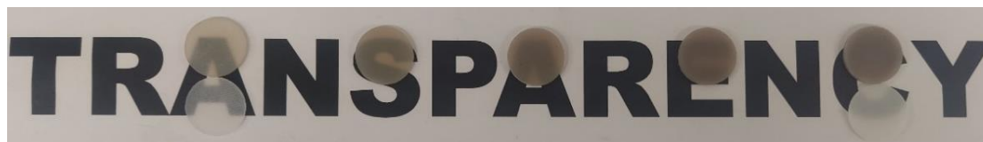
Figure 6.1. Digital image PUs synthesized using BHET-m (top) and BHET-ref (down) as chain extender.
