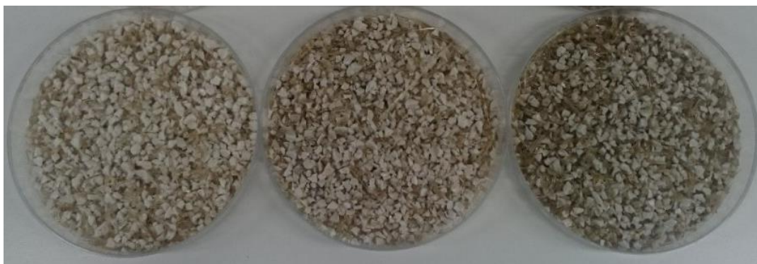
Figure 4.9. RPET blends with different compositions, from left to right 90u/10m, 80u/20m and 70u/30m.
