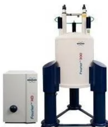
Figure 13. Bruker Avance 300 spectrometer.
