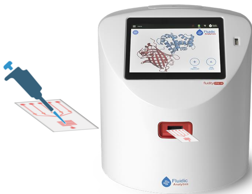
Figure 3.6. Fluidity One W system. The Fluidity One W system ( www.fluidic.com/product/fluidity-one-m/ ) is based on microfluidic diffusional sizing technology. Samples are deposited on a microfluidic chip and then introduced into the slot of the Fluidity One W system. After about 10-15 minutes, parameters such as apparent Rh are obtained.
